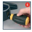
angle to the desired position. The mitre table features positive click stops at 0°, 15°, 22.5°, 30°, 45° and 50° for quick setting of common mitre angles.
